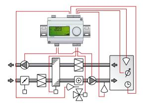
This control mode requires two sensors, "Supply air sensor " on AI1 and either "Room sensor" or "Extract sensor" on AI2.
