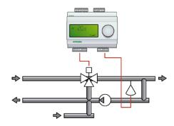
This control mode requires a sensor, "Supply water temperature", on AI1
