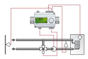
This control mode requires two sensors, "Supply temperature" on AI1 and "Outdoor sensor" on AI2.
