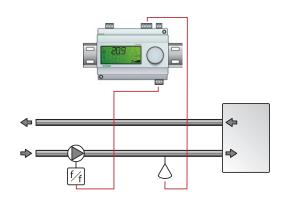
The output signal will increase when the pressure signal falls below the setpoint value.
