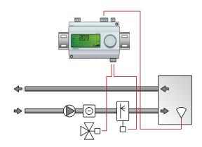
Humidification and dehumidification can be used simultaneously. A neutral zone can be set between humidification and dehumidification.
