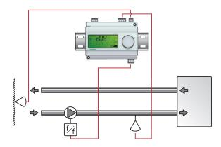
The output signal will increase when the pressure signal falls below the setpoint value.
